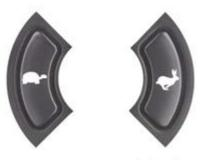
The user can adjust the machine's top drive speed to suit the environment. The currently selected top speed is shown on the Speedometer and can be adjusted using the Increase Speed (Hare) and Decrease Speed (Tortoise) buttons.
